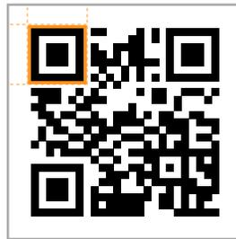
Once all the blocks in an image are identified, it then looks for known barcode patterns to filter the barcode locations. For instance, QR codes are characterized by a distinct square target in three of the four corners. Each square target in the corner consists of two blocks: a solid square in the middle of a hollow outer square. The cross-sectional thickness of the outer square, the gap and the width of the solid center square has the ratio of 1:1:3.
