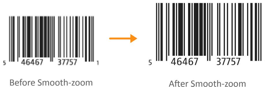
Smoothing a barcode that is lacking contrast or pixel density must be done intelligently and an appropriate zoom level should be employed in the barcode reader software. So, you can imagine that whenever smoothing is implemented, speed is sacrificed. Just as you want to avoid deskewing, you'll want to avoid smoothing too.
